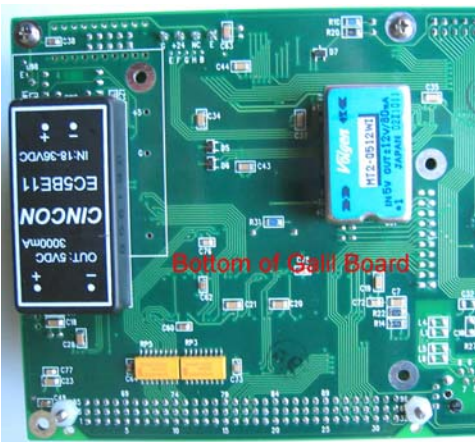
Bottom of Galil board showing plastic nuts
